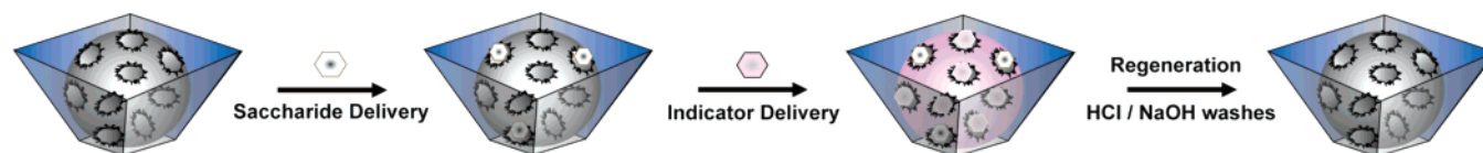
Figure 4. General scheme of the indicator uptake assay: saccharide (represented as white hexagons) is introduced to the RBRs in each of the pyramidal pits in the first step, followed by indicator (represented as pink hexagons) in the second step. Saccharide and indicator are then removed from the RBRs using acid and base washes.
